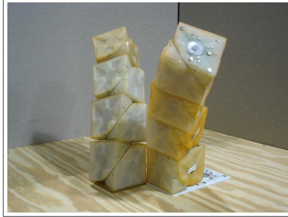
**Figure 2.16.** The self-replicating modular robot of Zykov et al.
